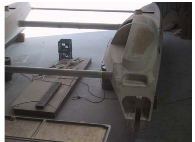
RADICAL BAY 8000 PHOTO UPDATE AS AT 27TH FEBRUARY 04. MATERIALS TO DATE $39,028.00 AND HOURS APPROXIMATELY 2000. SHE IS MOSTLY FAIRED AND WILL BE PAINTED SOON. INTERIOR FAIRED AND BEING PAINTED NOW.
