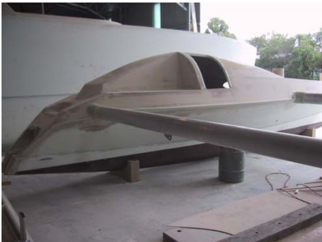
RADICAL BAY 8000 PHOTO UPDATE AS AT 27TH FEBRUARY 04. MATERIALS TO DATE $39,028.00 AND HOURS APPROXIMATELY 2000. SHE IS MOSTLY FAIRED AND WILL BE PAINTED SOON. INTERIOR FAIRED AND BEING PAINTED NOW.
