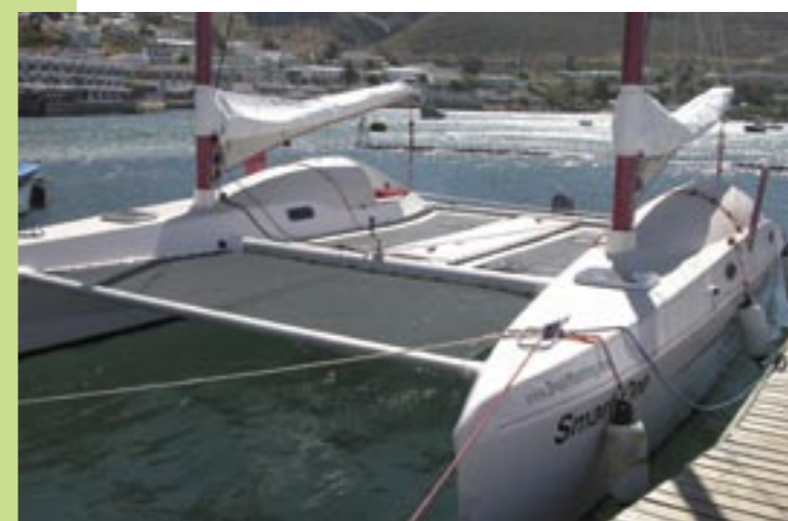
Top: The small outboard motor, attached to a pivoting 2m-long marine-grade aluminium tube, is lowered to the correct height and retained by two wires fixed to the underside of the aft beam. Left: As no rigging is required to support the free-standing carbon fibre rotating masts, the space between hulls is free of obstructions.
