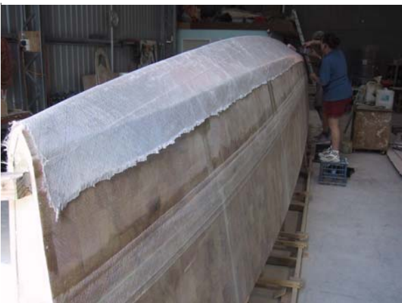
Joins and taped and bottom glassed.
