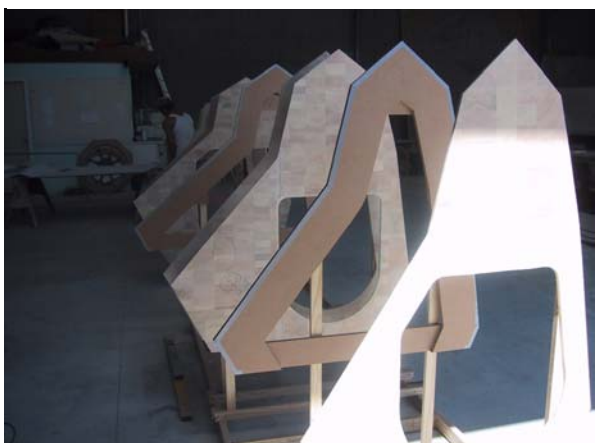
Bulkheads & temp. frames for 1st hull standing
