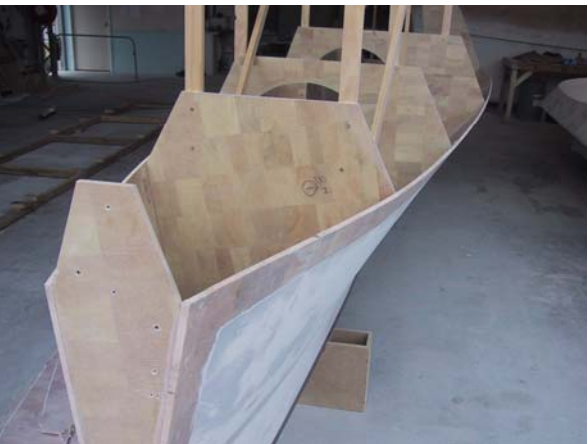
High Build undercoat sanded back.
