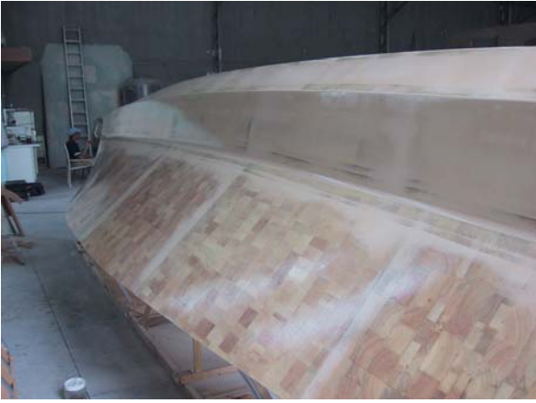
Fairing with Microlight fibres
