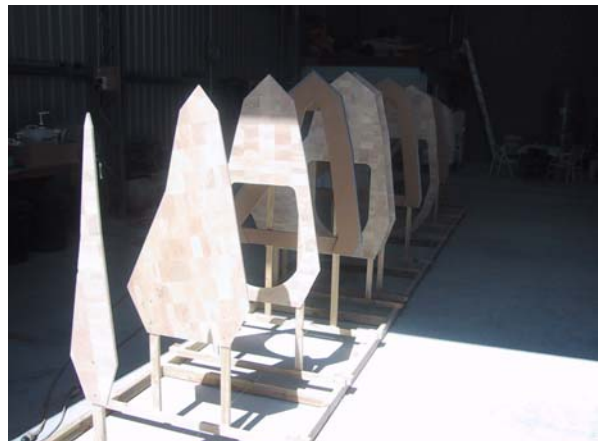
Bulkheads & temp. frames for 1st hull standing
