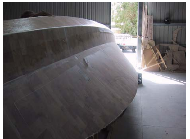
Note some pics show peel ply still attached
