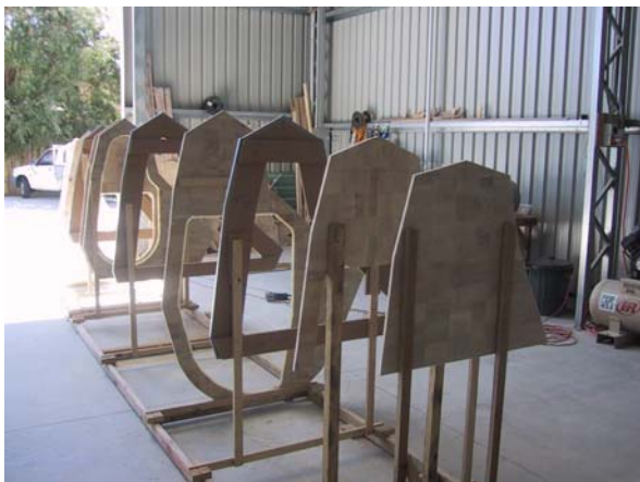
Bulkheads attached to strongback
