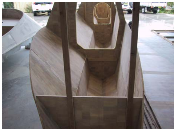
First hull turned over—note flared chamfer.
