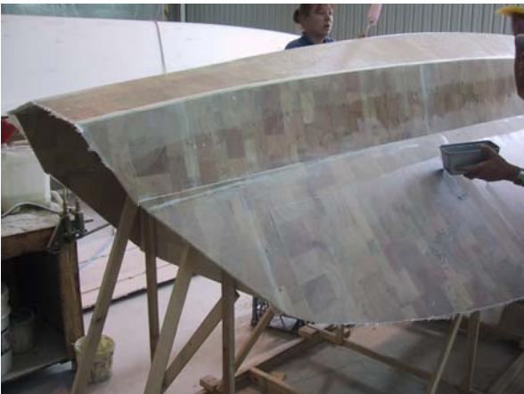
Joins and taped and bottom glassed.
