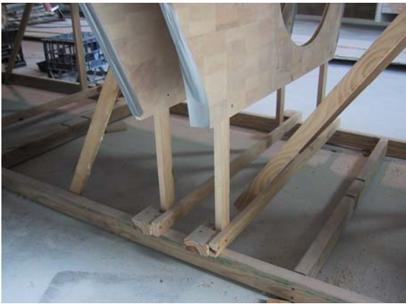
Bulkheads attached to strongback
