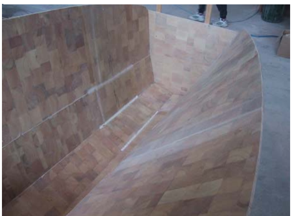
First hull turned over—note flared chamfer.
