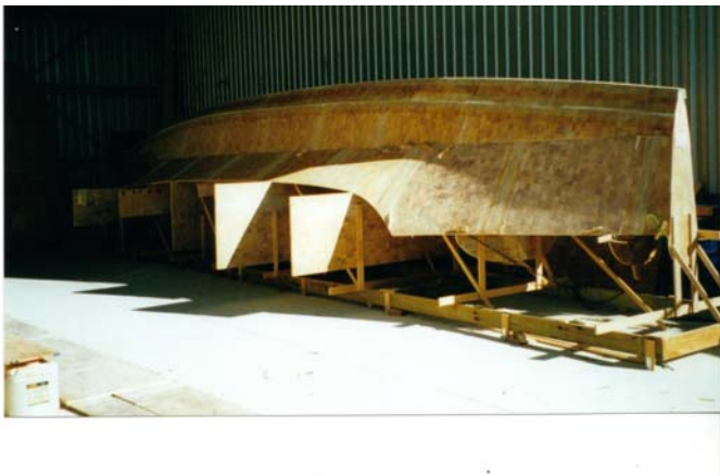
The chamfer panel is surface cut on one side to get the curved shape
