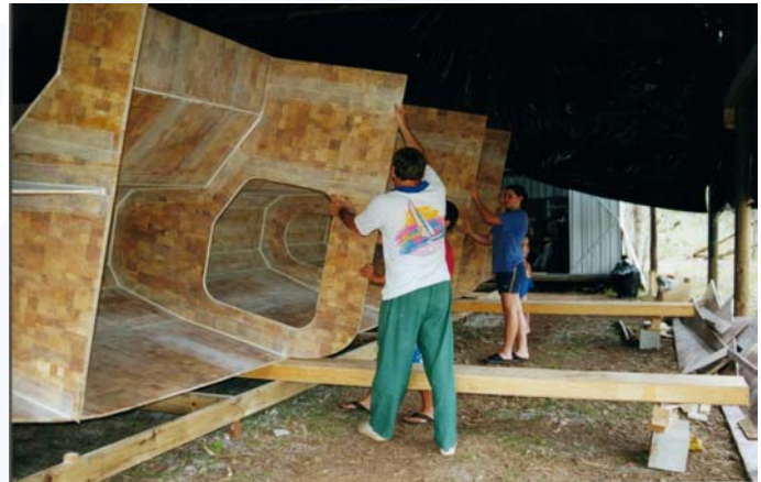
Turning the first hull. Small sections make the handling very easy, no expensive cranes required, just a few friends.
