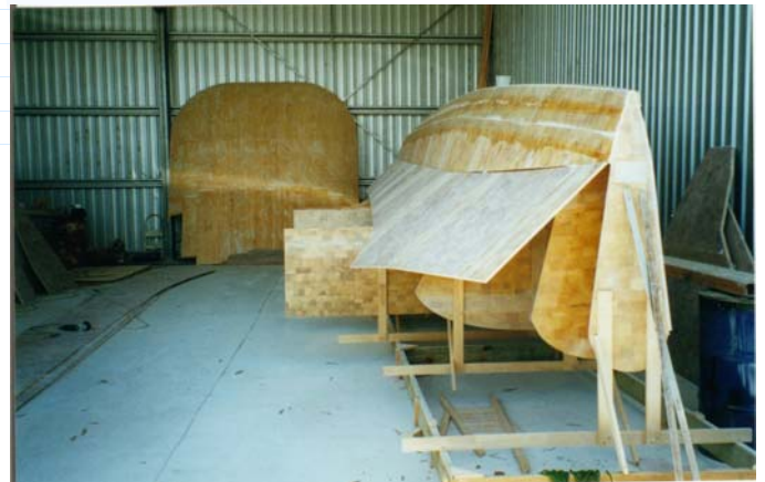
More hull panels fitted
