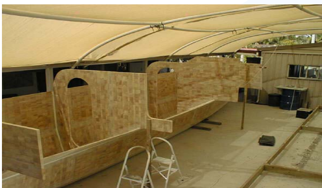
Hull turned with bulkheads taped in, now the second hull starts.
