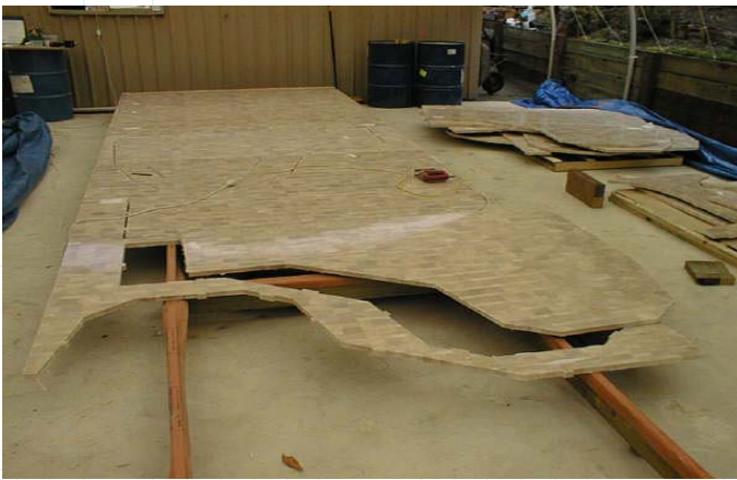
The Pre-cut kit arrives, the 8 x 4 panels are joined (pre-scarfed), the pieces are separated by cutting tags that keep the sheet together
